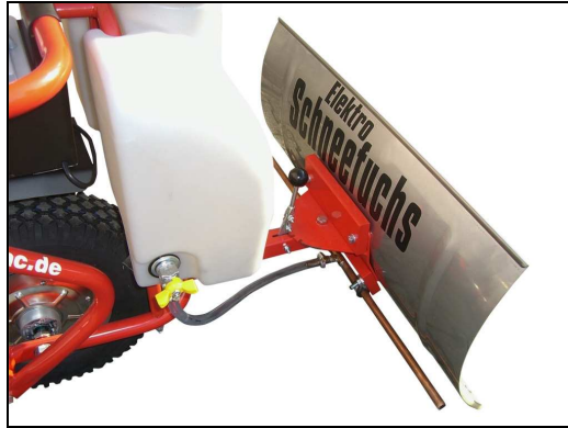
optional with liquid de-icing tank 13ltr. with spraying system
